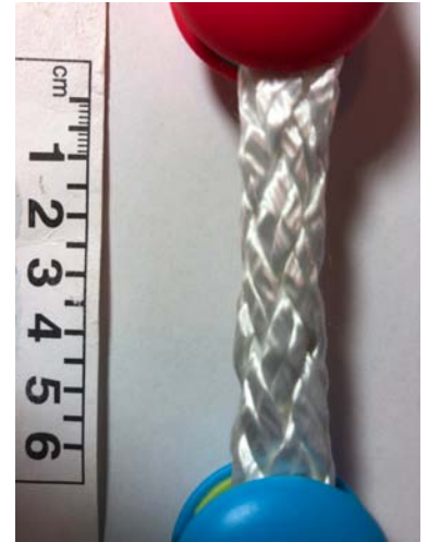
Figure 3a. Core of kernmantle rope in ‘neutral’ state (no tension or compression).
